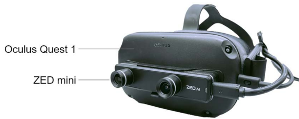
Fig. 3 Augmented reality head-mounted display device implemented with Oculus Quest first generation and ZED mini in this work
