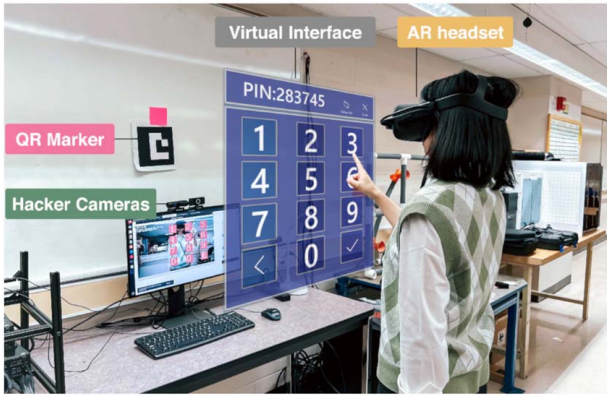
Fig. 5 The setup of password inference attacks in the MR system is illustrated
